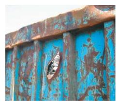
Scrap. A container made of a "mild steel" has cracked due to its poor resistance to wear, dents and blows. Not an attractive sight.
