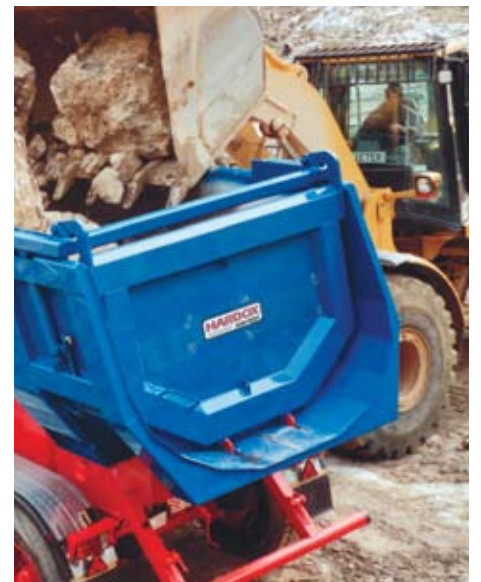
A truck body made of HARDOX wear steel is more durable due to the unique combination of hardness and toughness. Increased load-carrying capacity with unchanged weight results in better overall economy.
