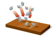
In impact wear, the aggregate rocks hit the surface of the wear component at various angles. A harder grade of HARDOX will deliver a longer service life here as well.
