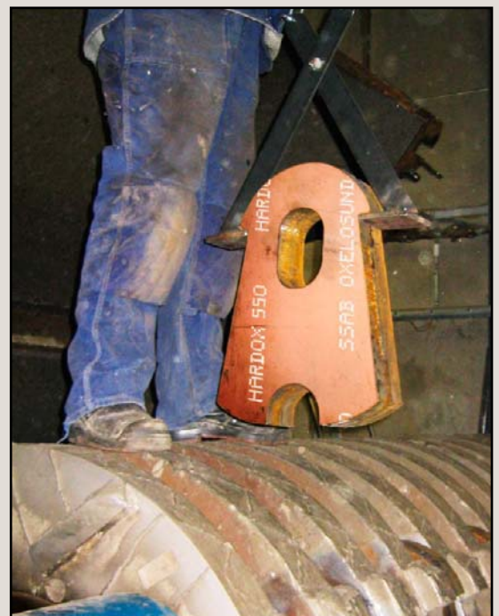
A hammer made of HARDOX 550 is inserted into a crusher
