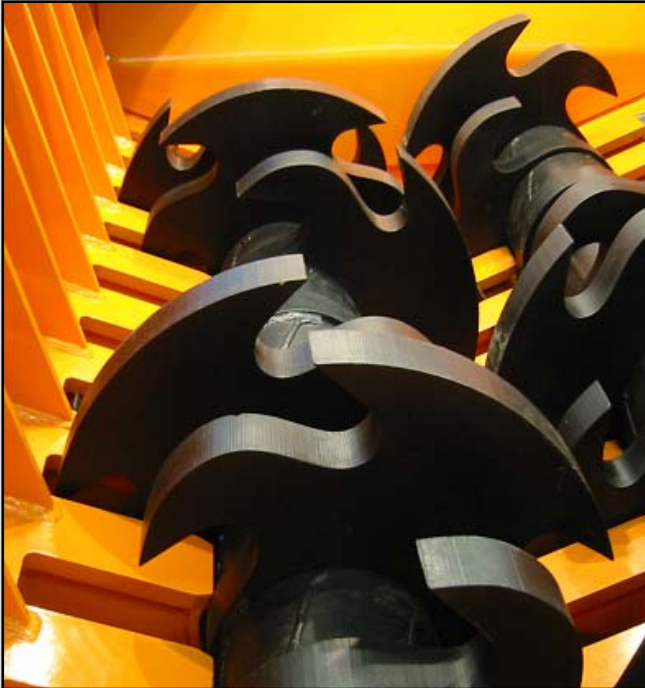
A shredder from M&H with HARDOX in the knives and liner plates
