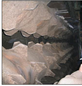
Before composting, the material needs to be turned and fragmentized. In this machine Hardox 600 are tested as blade material.
