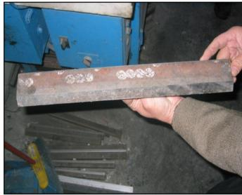
Materials as plastics are fragmentized with cutter machines. Linear plates of Hardox 450, axes made of Hardox 400, cutters and anvils made of Hardox 600.
